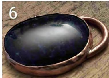
Polished up using a rotary tool and felt wheels, with a little polishing compound. A, B, and C are other views.
